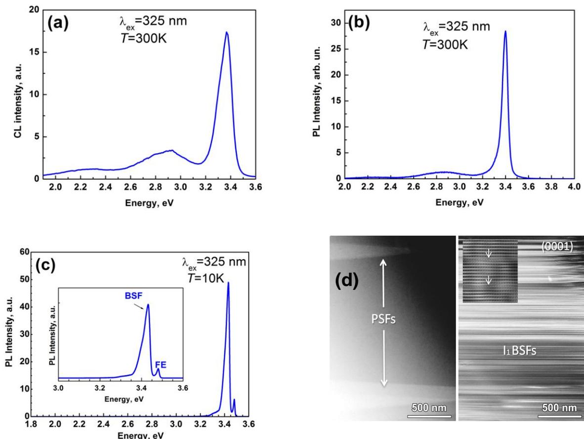
**Figure 2.** Luminescence of the studied material: RT CL (a) and PL (b) spectra, and a low-temperature PL spectrum dominated by the emission of excitons bound at BSFs with the inset showing the details of ‘edge’ PL (c). Image (d) shows TEM images of cross-sections of 1.5 mm-thick thick sample with prismatic stacking faults (PSFs, left image) and BSFs (right image), the inset shows a high-resolution TEM image of BSFs.
