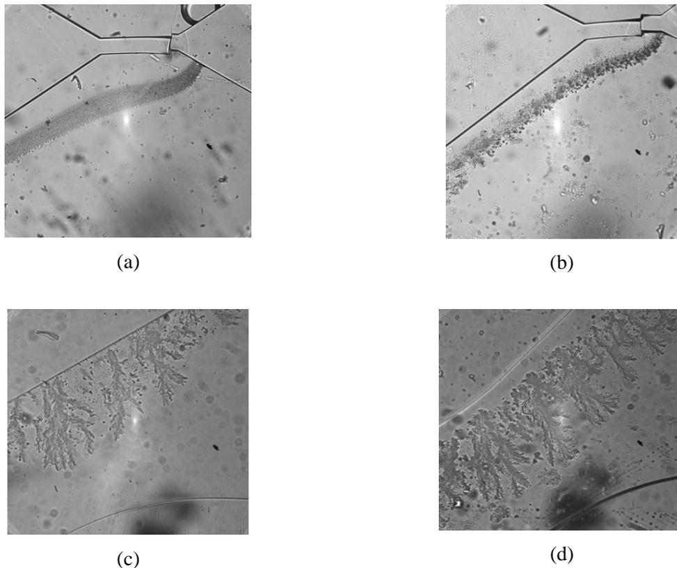
**Figure 3.** Formation of calcium phosphates in a microfluidic device at different concentrations of  $\text{CaCl}_2$ : (a) 0.2%, (b) 0.4%, (c) 0.6%, (d) 0.8%
