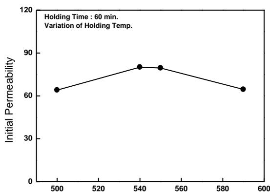
**Figure 1.** The variation of initial permeability with annealing temperature.
