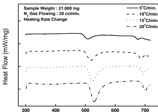
**Figure 3.** The Results of DSC analysis of amorphous FeSiBNbCu alloy at different heating rates.
