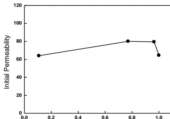
**Figure 4.** The variation of initial permeability of FeSiBNbCu alloy on volume fraction of bcc-Fe(Si) phase( $f_c$ ).
