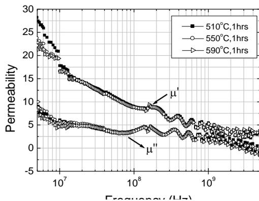
**Figure 5.** The complex relative permeability curve at various annealing conditions of FeSiBNbCu alloy.
