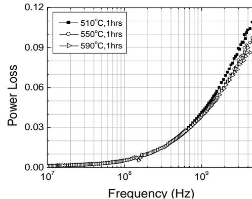
**Figure 6.** The EM wave absorption curve at various annealing conditions of FeSiBNbCu alloy.
