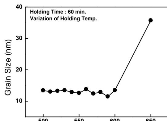
**Figure 2.** The variation in average grain size with annealing temperature.
