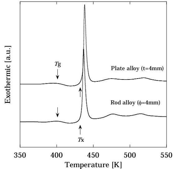
**Figure 2.** DSC curves for the  $\text{Ca}_{48}\text{Mg}_{27}\text{Cu}_{25}$  bulk metallic glasses.
