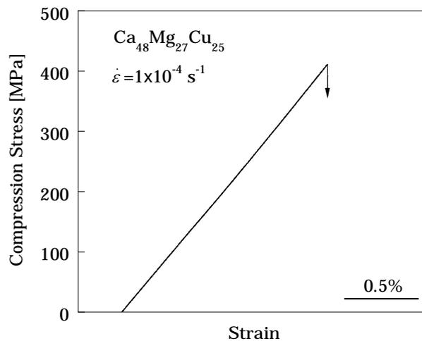
**Figure 3.** Compressive stress-strain curve for the  $\text{Ca}_{48}\text{Mg}_{27}\text{Cu}_{25}$  bulk metallic glass.
