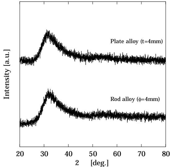
**Figure 1.** X-ray diffraction patterns for the  $\text{Ca}_{48}\text{Mg}_{27}\text{Cu}_{25}$  bulk metallic glasses.
