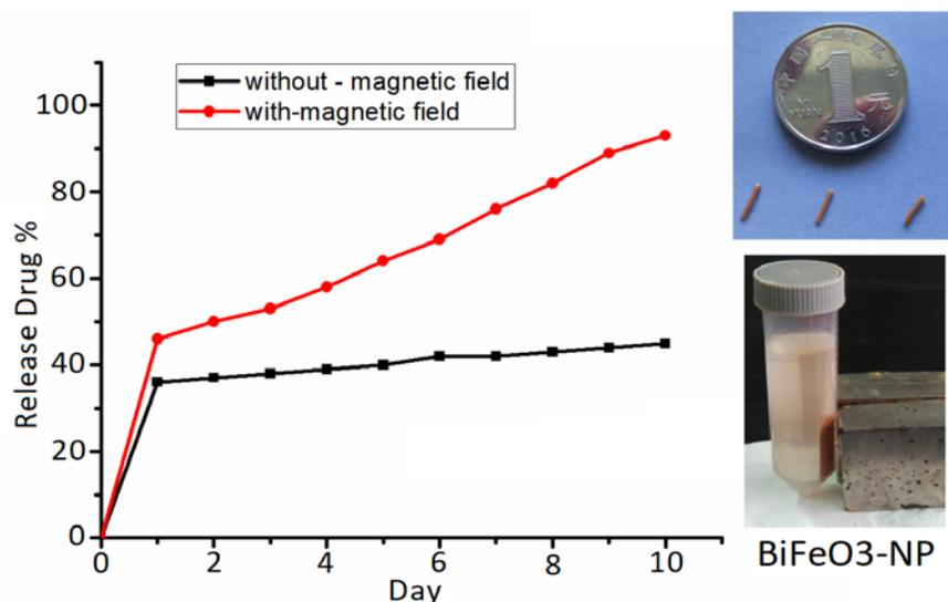
**Figure 6.** Drug release percentage from spacer (fiducial) with applying a magnetic field and without magnetic field.
