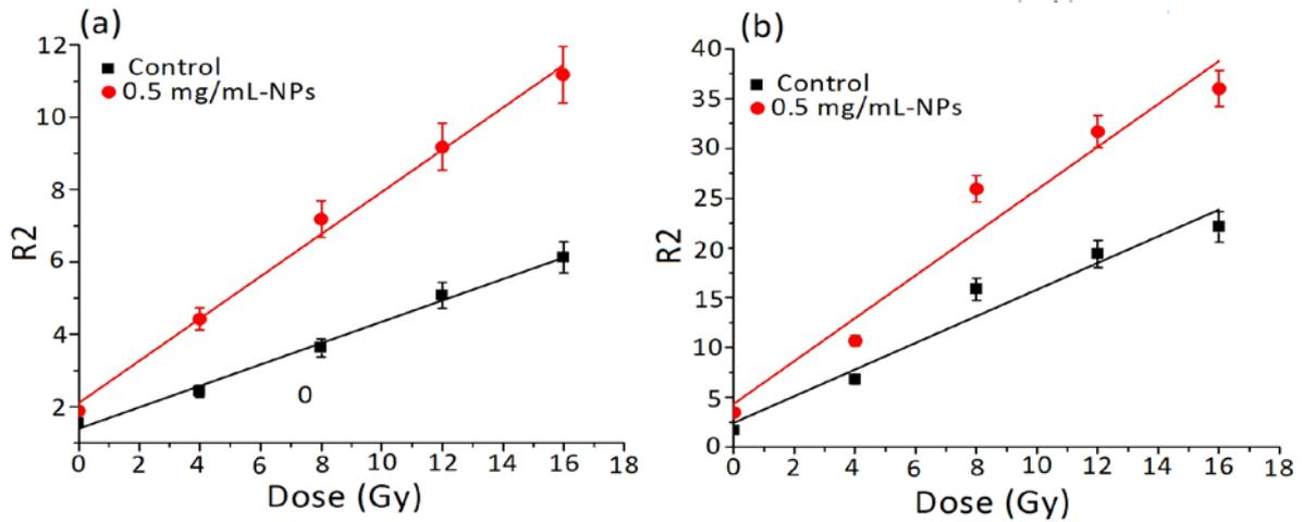
**Figure 3.** Gel dosimetry (a) dose response curves for gel pure and gel+BiFeO<sub>3</sub>-Np irradiated at energy of 160 keV. (b) At average energy of 380 keV.
