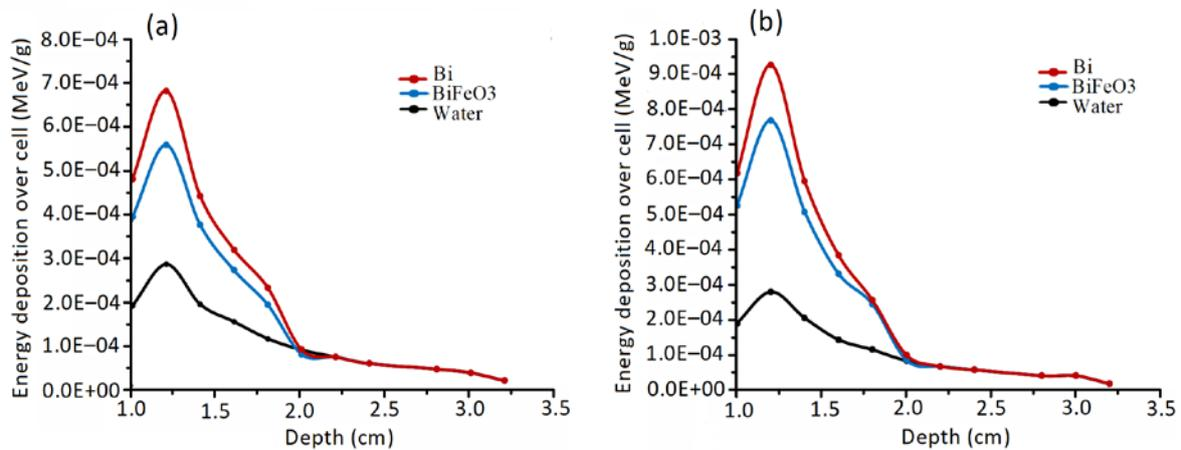
**Figure 5.** Energy deposition for bismuth and bismuth ferrite nanoparticles as dose enhancement agent (a) for 7mg and (b) for 15 mg.
