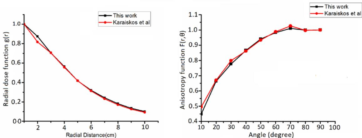
**Figure 4.** Comparison of radial dose function and anisotropy function of I-125, Selectseed 130.002 from the study and Karaiskos *et al* [13].
