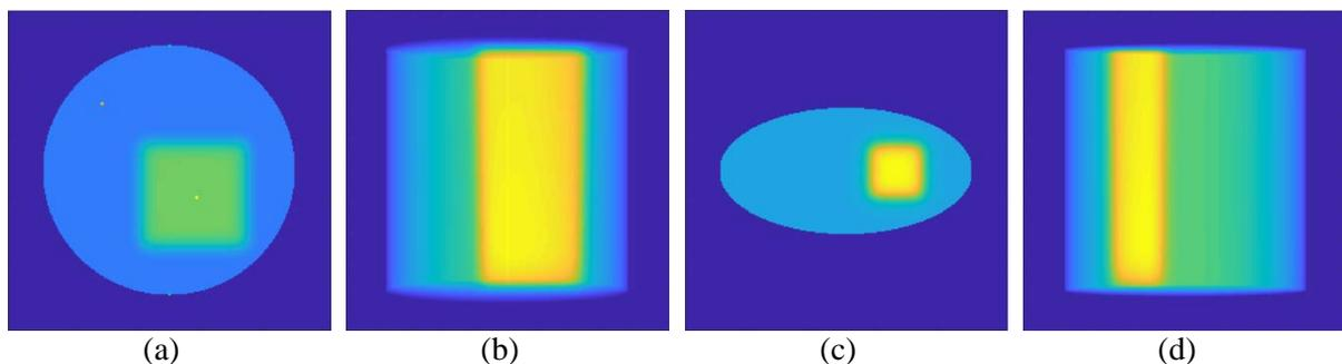
**Figure 1.** Defected cylindrical phantom: (a) central axial slice and (b) projection image; Elliptical phantom: (c) central axial slice and (d) projection image.
