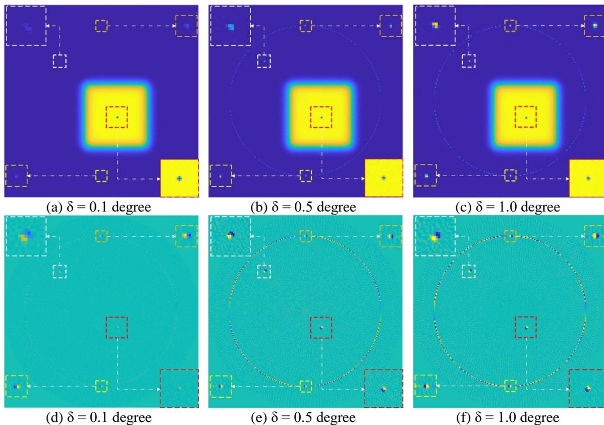
**Figure 2.** Reconstructed images with zoomed details when the angles are mismatched by (a) 0.1 degree, (b) 0.5 degree and (c) 1.0 deg. Difference maps with zoomed details between the perfect matching resultant image and (a) (b) and (c) are shown in (d) (e) and (f) respectively.
