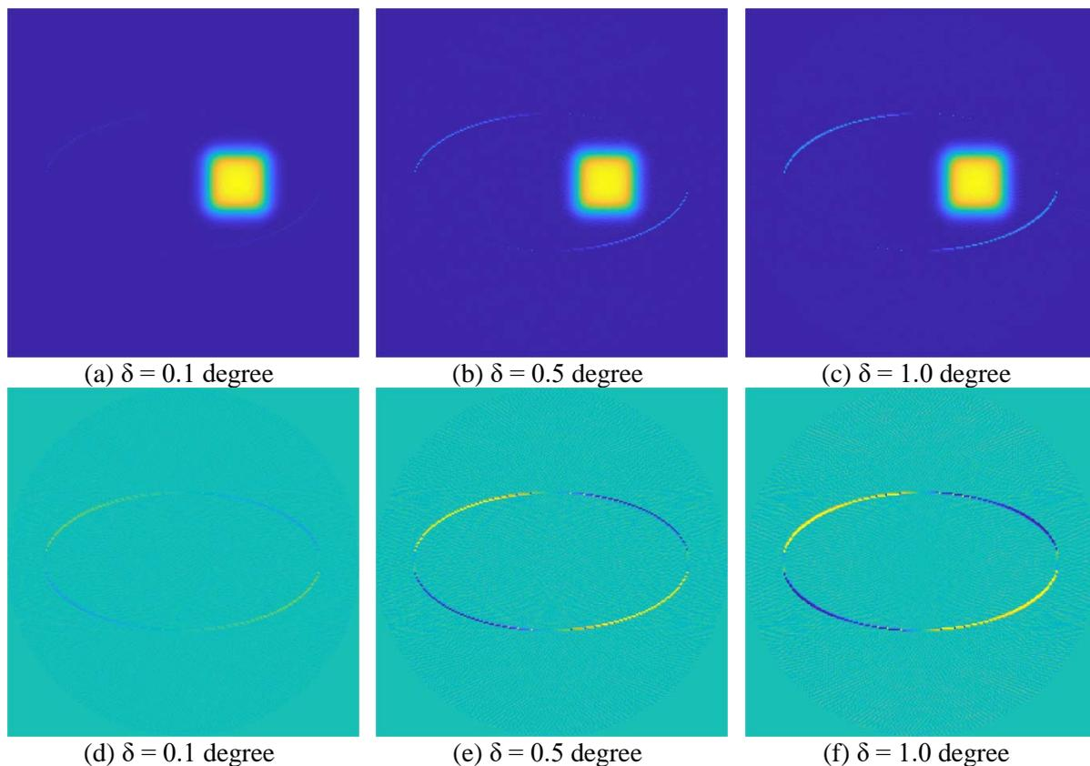
**Figure 3.** Reconstructed images with zoomed details when the angles are mismatched by (a) 0.1 degree, (b) 0.5 degree and (c) 1.0 degree. Difference maps with zoomed details between the perfect matching resultant image and (a) (b) and (c) are shown in (d) (e) and (f) respectively.
