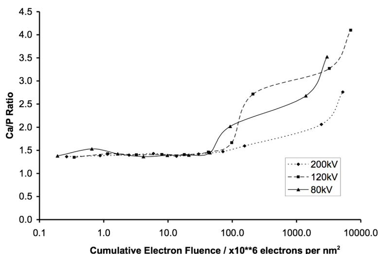
Figure 2. EDX Ca/P ratio in HA plotted as a function of electron fluence for three different accelerating voltages: 80, 120 and 200 kV.
