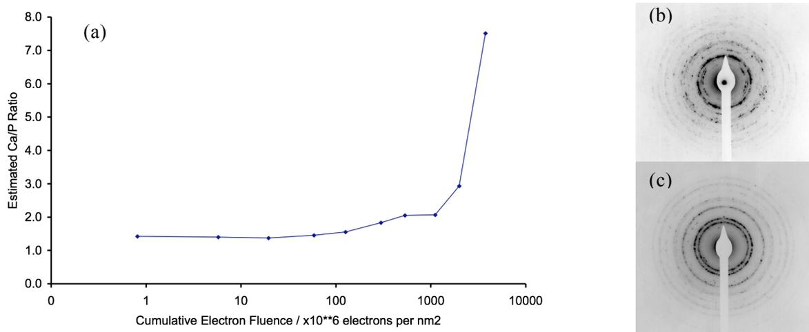
Figure 1. (a) EDX Ca/P ratio in HA plotted as a function of electron fluence. Selected area electron diffraction patterns at (b) low total fluence < ca. 10<sup>8</sup> electrons/ nm<sup>2</sup> and (c) high total fluence > 10<sup>8</sup> electrons/ nm<sup>2</sup>.
