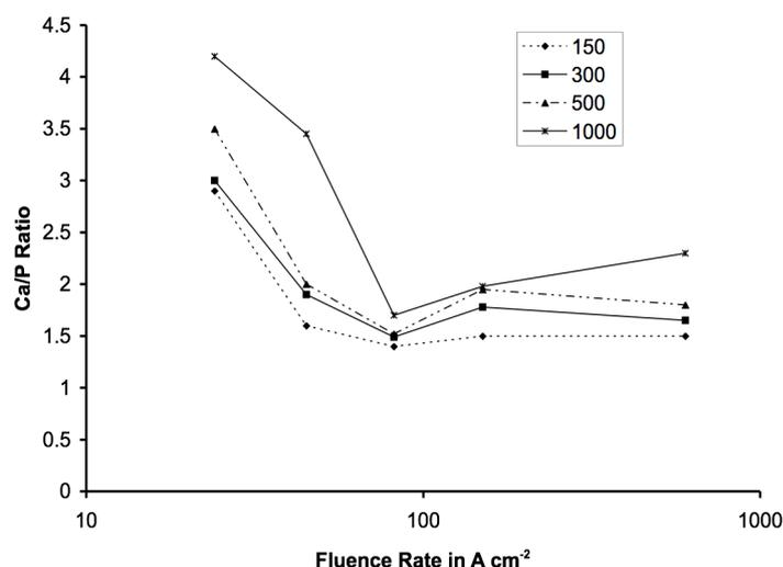
Figure 3. (a) EDX Ca/P ratio in HA plotted as a function of electron fluence rate (in Amps per  $\text{cm}^2$ ) for four different total fluences : 150, 300, 500 & 1000 electrons  $\text{nm}^{-2} \times 10^6$ .
