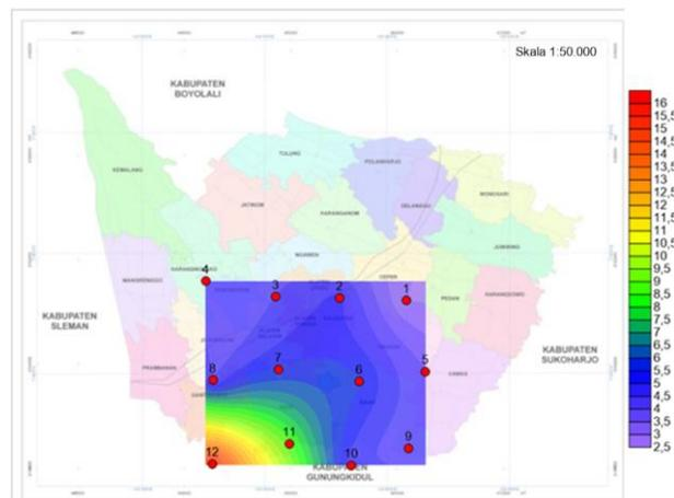
**Figure 5.** The microzonation of seismic vulnerability index ( $K_s$ ) in the southern area of Klaten regency
