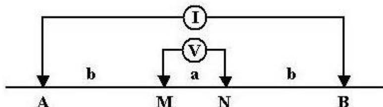
**Figure 2.** Schlumberger configuration of geoelectric methods
