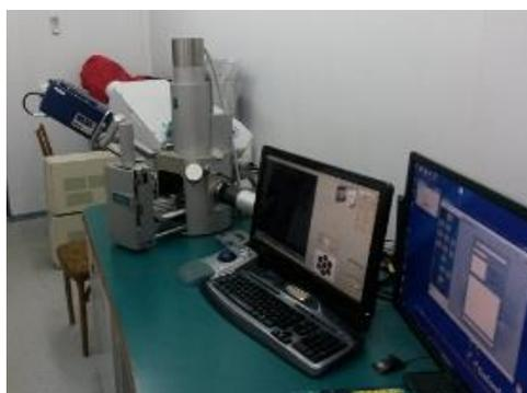
**Figure 4.** The analytical complex of the scanning electron microscope “VEGA II LMU” Tescan, Czech Republic combined with the energy-dispersive X-ray spectrometer of the model INCA Energy 350
