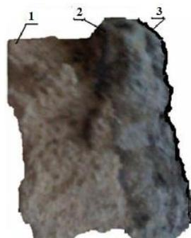
**Figure 2.** A sample of broken lining: 1 – a semi-sintered layer, 2 – a sintered layer, 3 – a slag layer
