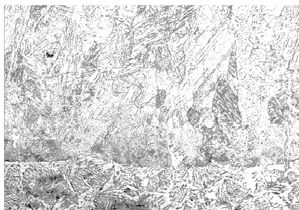
Figure 4. A structure of the transition zone “surfaced coat T590 - steel base (09G2S)”, \times 500 .
