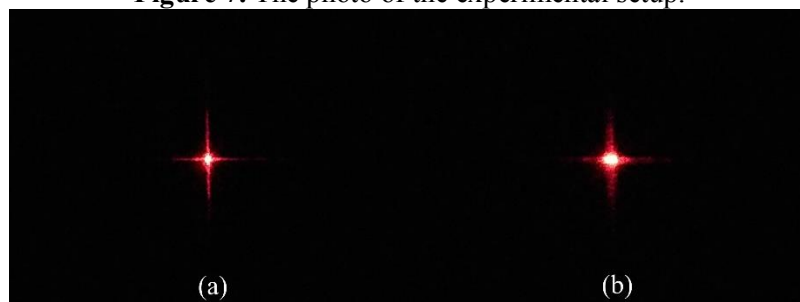
Figure 8. A focusing dot for a plane wave (a) and for a wave with 5\lambda defocusing aberration (b) without a CGH at the SLM.
