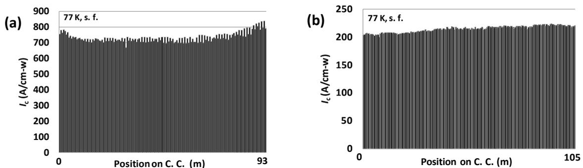
Fig. 2 Longitudinal  $I_c$  distributions at 77 K and self-field of (a) a 93 m long EuBCO with BHO coated conductor by conventional PLD method and (b) a 105 m long EuBCO with BHO coated conductor by in-plume (plane-plume) PLD method.
