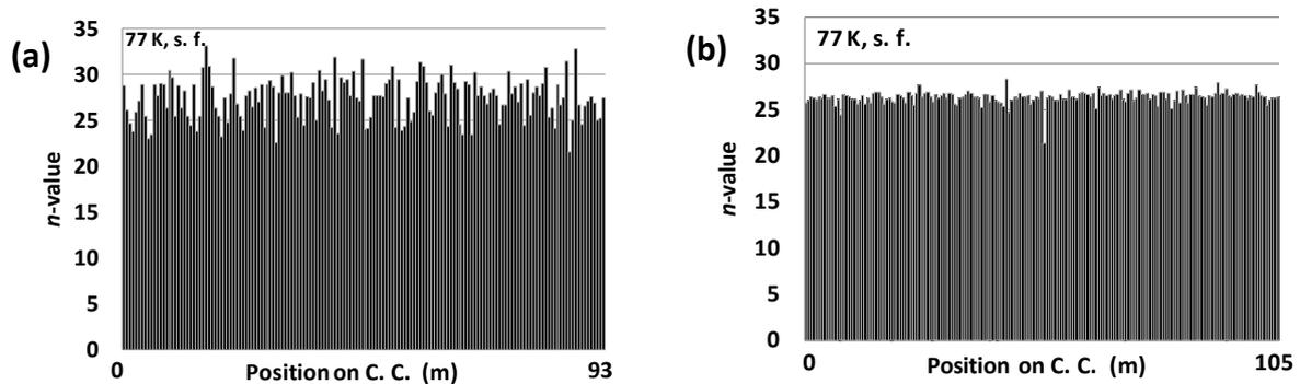
Fig. 3 Longitudinal  $n$ -values at 77 K and self-field of (a) a 93 m long EuBCO with BHO coated conductor by conventional PLD method and (b) a 105 m long EuBCO with BHO coated conductor by in-plume (plane-plume) PLD method.
