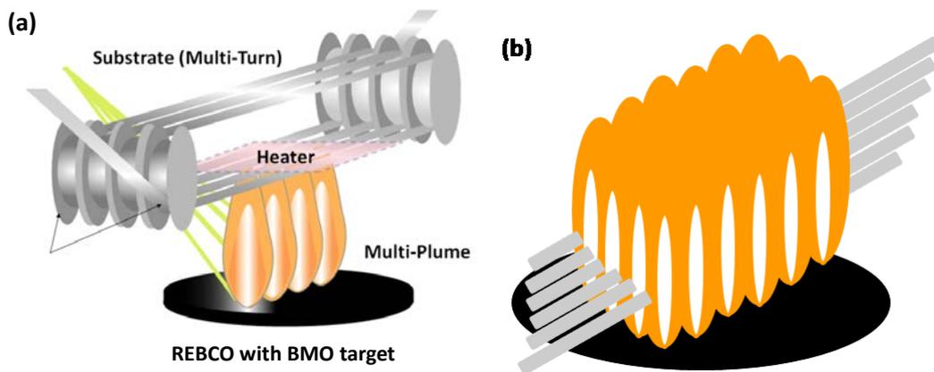
Fig. 1 (a) schematic diagrams of our conventional (out-of-plume) and (b) in-plume (plane-plume) PLD system.
