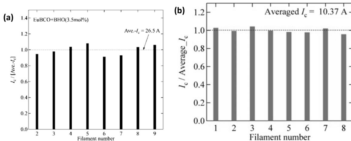
Fig. 4 Normalized  $I_c$  distributions of (a) 0.6 m long EuBCO with BHO coated conductor of 8 filaments of 440  $\mu\text{m}$  in width by conventional PLD method and (b) 0.6 m long EuBCO with BHO coated conductor of 8 filaments of 581  $\mu\text{m}$  in width by in-plume (plane-plume) PLD method.
