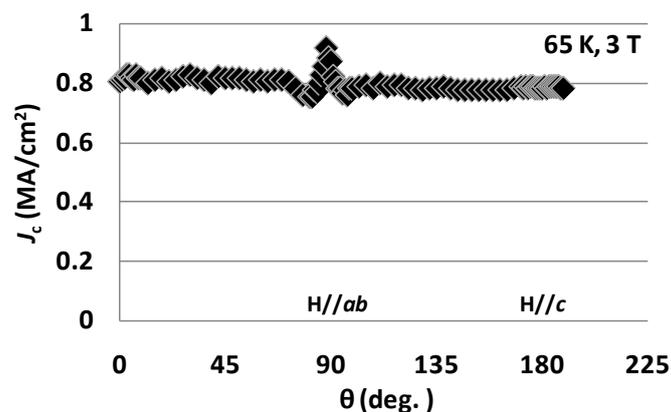
Fig. 5 Angular dependence of applied magnetic field of 3 T on  $I_c$  values for EuBCO with BHO coated conductor at 65 K by in-plume (plane-plume) PLD method.
