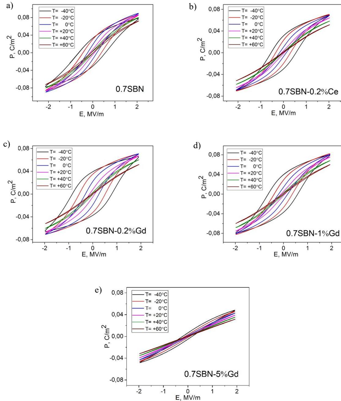
**Figure 2.** Ferroelectric hysteresis loops at some different temperatures for ceramic samples based on 0.7SBN (a), 0.7SBN-0.2%Ce (b), 0.7SBN-0.2%Gd (c), 0.7SBN-1%Gd (d) and 0.7SBN-5%Gd (e).
