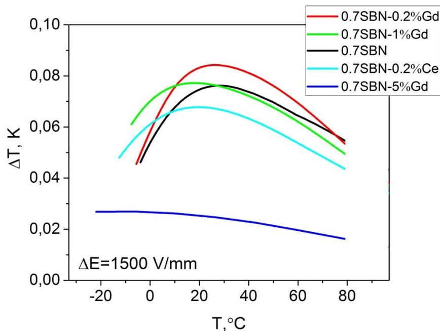
**Figure 4.** The temperature dependence of the electrocaloric effect.
