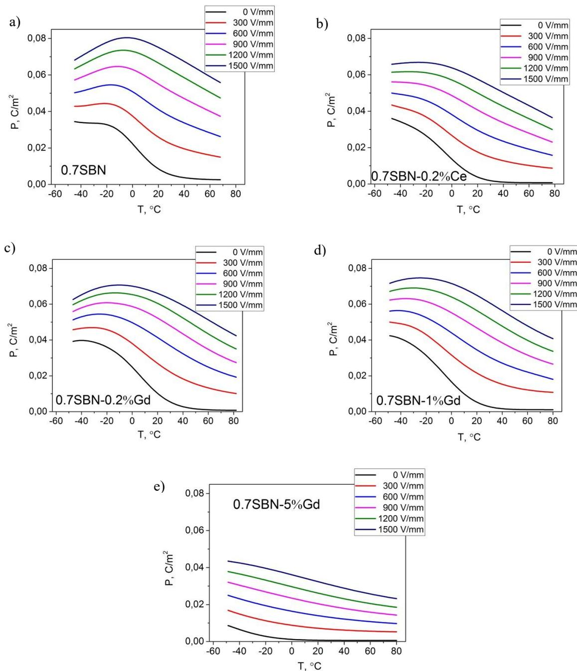
**Figure 3.** The dependence of electric polarization versus temperature at different electric field for ceramic samples based on 0.7SBN (a), 0.7SBN-0.2%Ce (b), 0.7SBN-0.2%Gd (c), 0.7SBN-1%Gd (d) and 0.7SBN-5%Gd (e).
