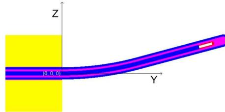
Fig. 4. Sabrina view of the source into the applicator (YZ plan at x= 0 source position 1)
