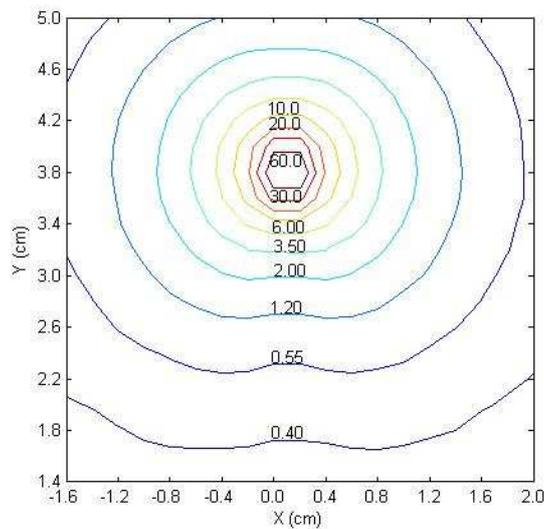
Fig. 5. Relative isodose curves (in %) around the applicator normalised in source centre
