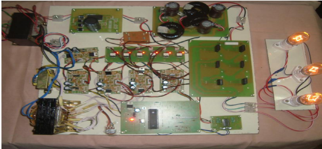
Figure 7. Experimental Output of EZ inverter
