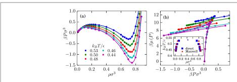
**Figure 4.** (a) Scaled pressure—density  $P-\rho$ , and (b) chemical potential-pressure  $\mu$ –P relations of an active LJ fluid at several temperatures  $k_BT/\epsilon$  and Péclet  $Pe=v_0/\sigma D_r=2.67$ . The inset shows the temperature—density gas—liquid binodals as obtained from direct coexistence simulations ( $\blacksquare$ ) and from equating  $\mu$  and P in the coexisting phases ( $\blacksquare$ ) of an active LJ fluid.
