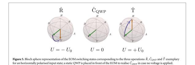
static QWP with  $\hat{C}_{QWP}$  in front of it. Now we have a balanced coin when no voltage is applied in the EOM and can switch to reflection or transmission by applying a positive or negative voltage  $U_0$ , respectively (figure 5).
