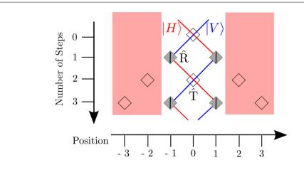
**Figure 3.** Illustration of how the spread of the walker's external state is limited via polarisation switching; a reflection  $\hat{R}$  is represented by a grey box and switches the horizontal (red lines) into vertical (blue lines) polarisation and vice versa. The transmission operation  $\hat{T}$  is represented by a white box leaving the polarisations unchanged. Note that in the setup the spatial position is in the experiment mapped into the time domain.
