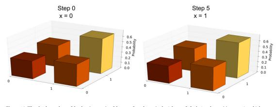
**Figure 18.** The absolute values of the density matrix of the transferred state in the 0th step (left plot) at the position x = 0 and 5th step at the position x = 1 (right plot) of a state transfer with a periodicity of 5 steps (scheme illustrated in figure 17); the observed fidelity  $F(\rho_0, \rho_5)$  is 99.4%.
