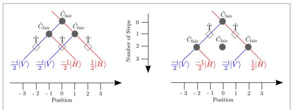
**Figure 13.** Illustration of the implementation of the states  $|\Psi_{VVHH}\rangle$  (left figure) and  $|\Psi_{VHVH}\rangle$  (right figure) with the three-stateswitching scheme for an horizontally polarised input state.
