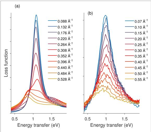
Figure 1. Loss functions for 2H- $Cu_{0.2}NbS_2$  based on (a) TDDFT calculation and (b) EELS experiment for several momentum transfers indicated in the legends.
