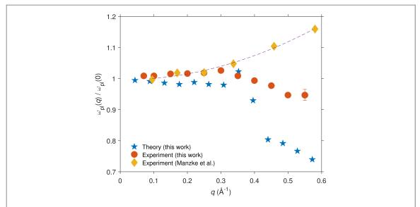
**Figure 3.** Plasmon dispersion for  $Cu_{0.2}NbS_2$  as a function of q for experiment, theory, and compared to published results for  $NbS_2$  [10]. The dashed line is a quadratic fit to the data points of [10].
