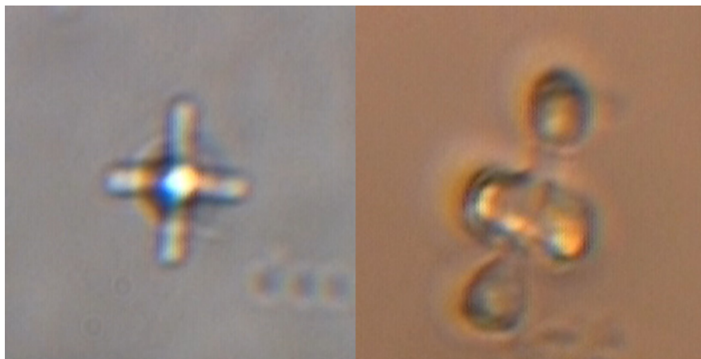
Figure 4. Bright field microscope image of a microfabricated paddle-wheel in unpolymerized resin (left) and after acetone wash (right).
