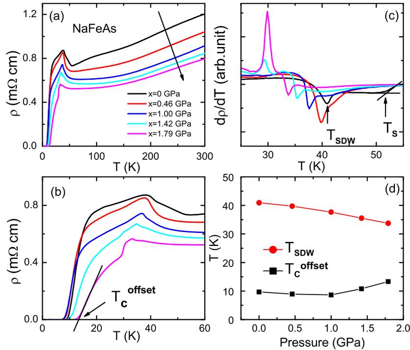
**Figure 1.** (a) Temperature dependence of in-plane resistivity for NaFeAs under different pressures. The arrow indicates the direction of the increasing pressure. (b) Expanded plot of the temperature dependence of resistivity under various pressures around  $T_c$ . (c) The derivative of the in-plane resistivity  $d\rho/dT$  and the criteria by which we infer  $T_s$  and  $T_{SDW}$ . (d)  $T_c$  and  $T_{SDW}$  as a function of pressure for the parent compound NaFeAs.
