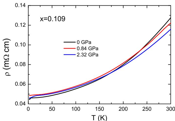
**Figure 5.** Temperature dependence of in-plane resistivity for heavily overdoped non-superconducting crystal  $\text{NaFe}_{0.891}\text{Co}_{0.109}\text{As}$  under various pressures.
