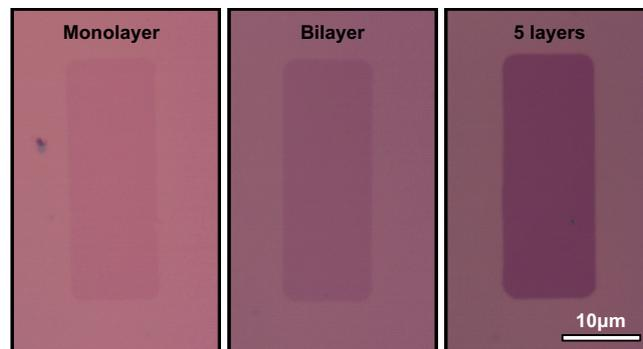
**Figure 2.** Optical images of graphene samples after the etch process from left to right, monolayer, bilayer and five layers.
