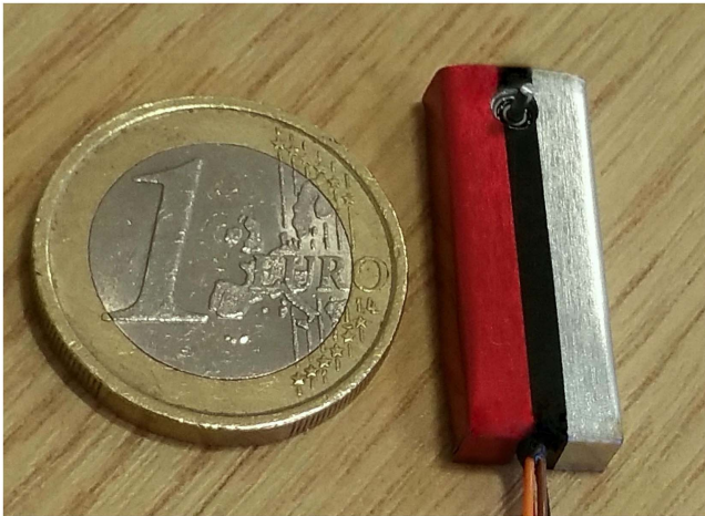
Figure 1. Low power consumption and light weight (0.7 g without the cover) mini rotary actuator (MiRA) with on board contact-less position and force sensors with overall measurements of 25.0 \times 9.0 \times 3.5 mm.
