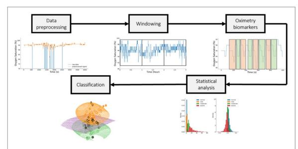
**Figure 19.** Flowchart for continuous oximetry time series analysis. Source: Adapted from: Behar *et al* 'Digital oximetry biomarkers for assessing respiratory function: standards of measurement, physiological interpretation, and clinical use', npj Digital Medicine, 2021, https://doi.org/10.1038/s41746-020-00373-5 (CC BY 4.0).
