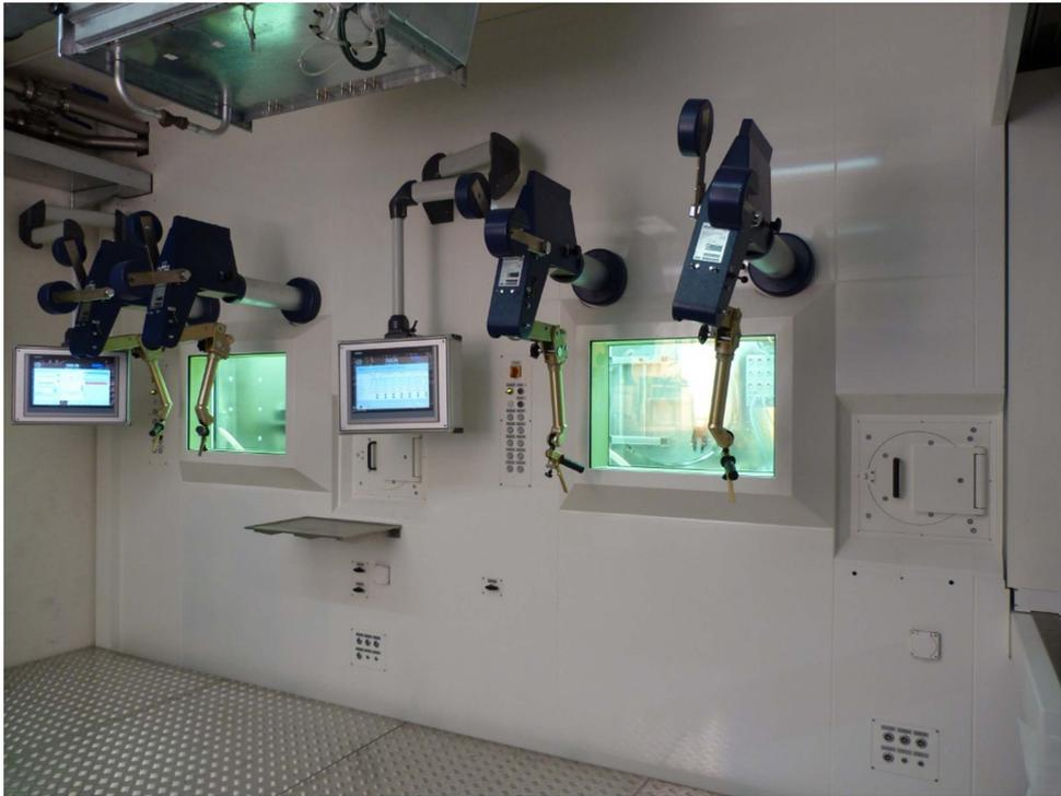
**Figure 9.** The alpha-gamma hot cell.
