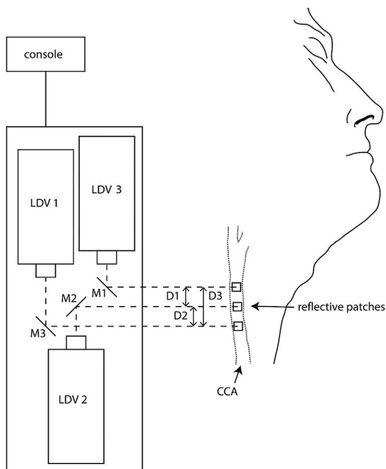
**Figure 1.** 3 laser Doppler vibrometer systems (LDV 1–3) mounted on a platform project 3 parallel low intensity laser beams by means of tunable mirrors (M1–3) on 3 equally spaced ( $D1-3$ , with  $D1 = D2$ ) reflective patches attached on a straight line along the trajectory of the right common carotid artery (CCA).
