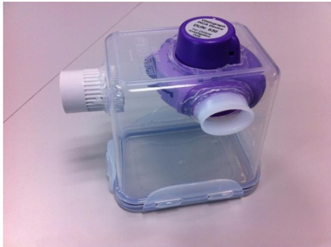
**Figure 2.** Airtight container with the Diskus™ inhaler placed inside and INCA device attached on top.
