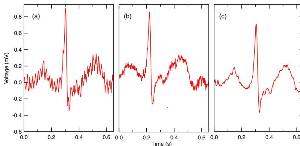
**Figure 11.** ECG measurement without ground connection (a), with ground connection (b) and with software filters (c).
