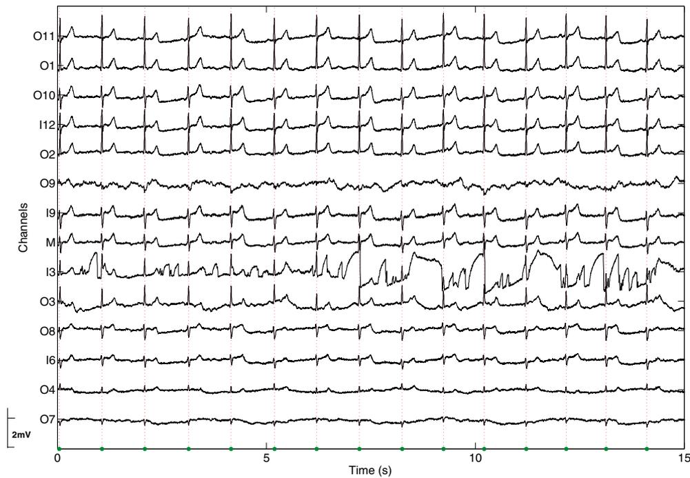
**Figure 8.** cECG time trace of all channels recorded over 15 s with QRS detection.
