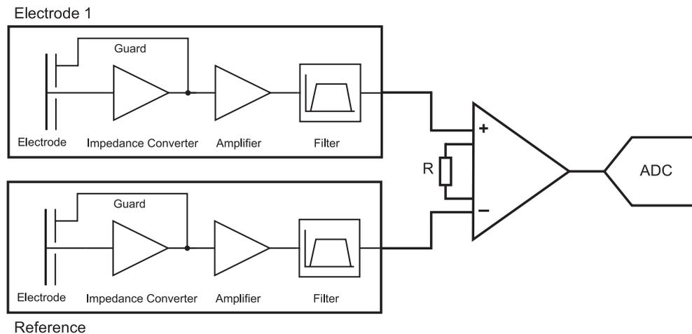
Figure 2. Sensor block diagram in differential configuration.
