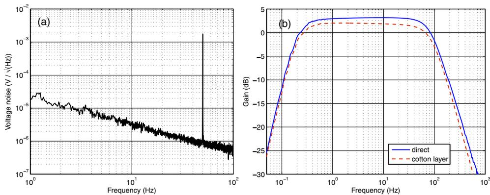
**Figure 3.** Voltage noise spectrum and frequency response of the capacitive sensor.
