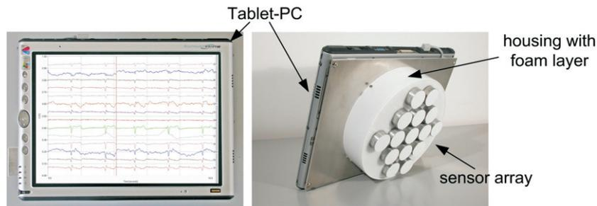
Figure 1. Tablet-PC-based multichannel ECG.
