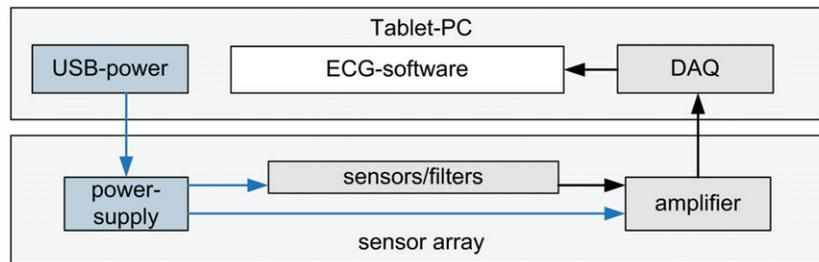
Figure 5. Signal flow and power distribution.
