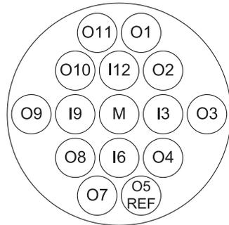
Figure 6. Sensor arrangement of the array (view to the body).
