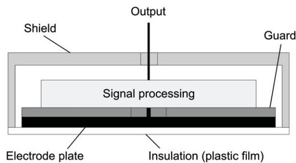
**Figure 4.** Sensor configuration (diameter: 30 mm, height: 15 mm).
