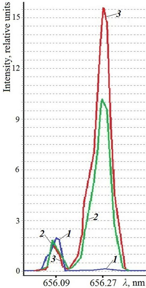
**Figure 2.** Spectra of a  $D_0$ - $H_0$  doublet. Pressure of added deuterium  $p_{D_2} = 0.05$  mbar. (1) no  $H_2O$  added; (2)  $p_{H_2O} = 0.05$  mbar; (3)  $p_{H_2O} = 0.1$  mbar. The both monochromator slit widths are of 0.01 mm.
