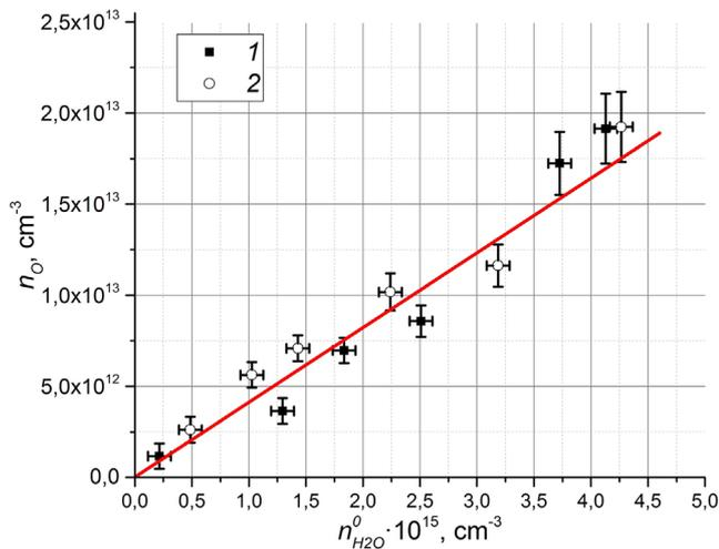
**Figure 3.** Concentrations of oxygen atoms measured using the lines at 777 nm (1) and 844 nm (2).
