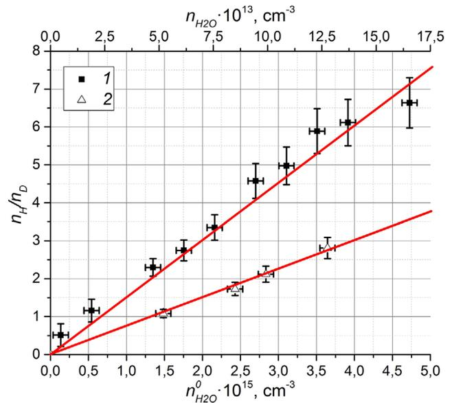
**Figure 5.** The  $n_H/n_D$  ratio for different amounts of deuterium. (1) The initial concentration of  $D_2$  in gas mixture  $n_{D_2} = 6.75 \cdot 10^{14} \text{ cm}^{-3}$ ; (2)  $n_{D_2} = 1.35 \cdot 10^{15} \text{ cm}^{-3}$ .
