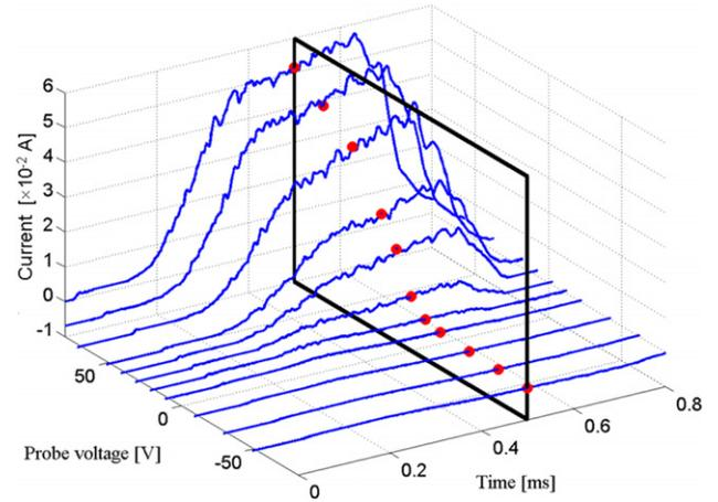
**Figure 2.** A slice is taken through the current versus time curves at a particular time (e.g. 0.5 ms shown here). The current values at that time, together with the voltages for each curve, are used to determine the  $I-V$  curve for that point in time.  $I-V$  curves, constructed in this way, were then used to obtain the EEDF and  $T_e$  and  $n_e$ .
