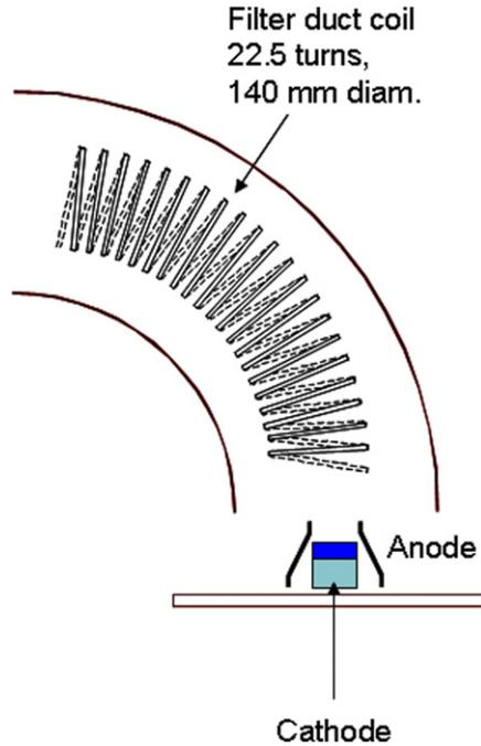
**Figure 1.** Schematic of one arm of the half torus, showing positions of the substrate, the magnetic filter and the cathode assembly.
