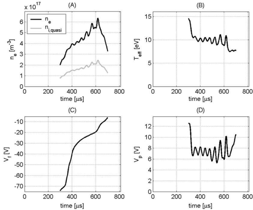
**Figure 4.** Plasma parameters,  $n_e$ ,  $n_i$ ,  $T_{\text{eff}}$ ,  $V_p$  and  $V_f$  over most of the pulse, 300–700  $\mu\text{s}$ .
