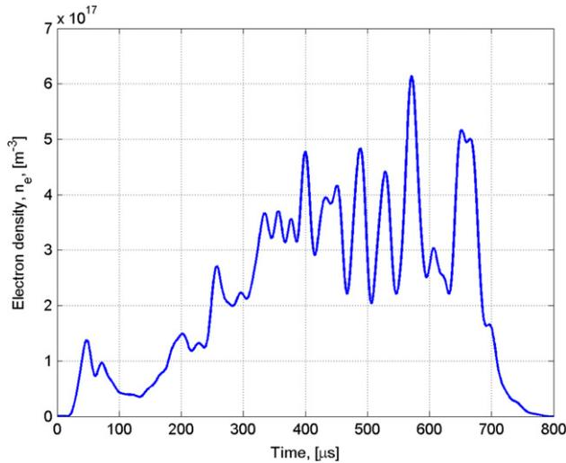
**Figure 5.** Average electron density measured using an 8 mm microwave interferometer.
