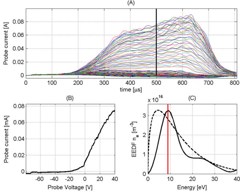
**Figure 3.** (a) The current curves for all probe voltages. (b) The  $I$ - $V$  curve using the data slice at  $500 \mu s$  (intercepted in (a)). (c) The EEDF (—), calculated from the  $I$ - $V$  curve shown in (b), compared with a Maxwellian distribution (- - -). The effective electron temperature for this time slice is  $9 eV$  and the electron density is  $7.5 \times 10^{17}$ .
