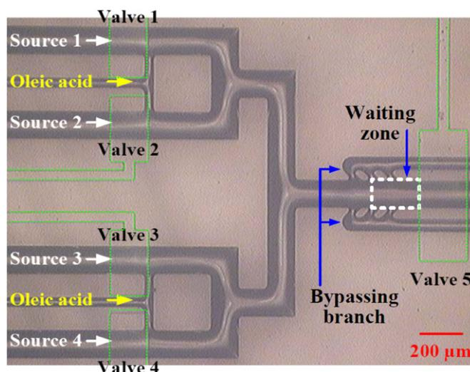
Figure 5. Photograph of a fabricated metering and coalescing PDMS device with four sources.
