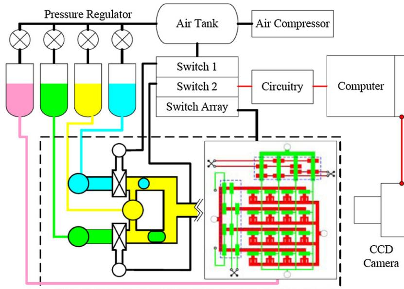
**Figure 7.** Experimental setup of the proposed random-access microarray.
