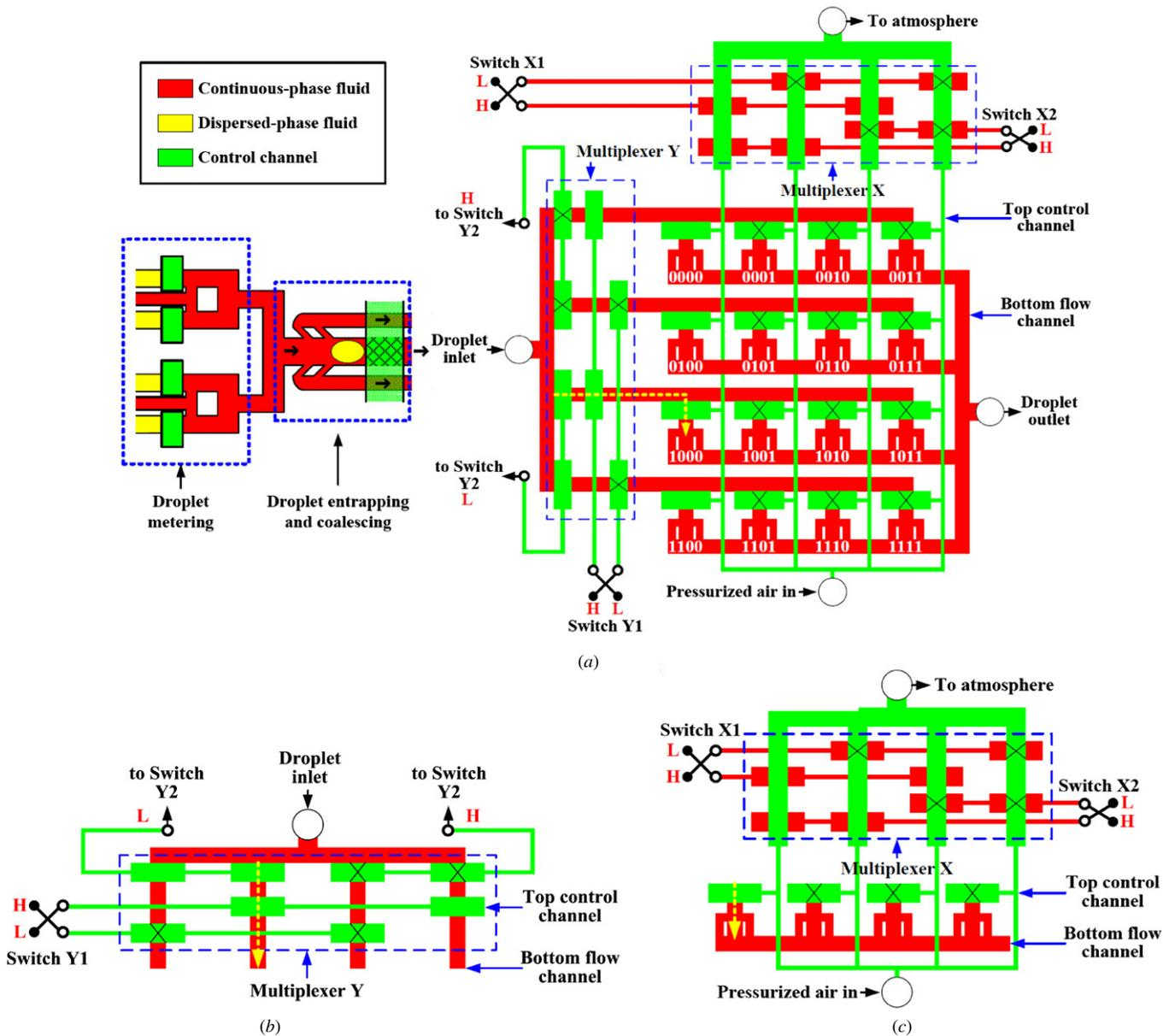
**Figure 1.** Schematic illustrations of (a) the proposed  $4 \times 4$  random-access microarray, (b) multiplexer Y and (c) multiplexer X.
