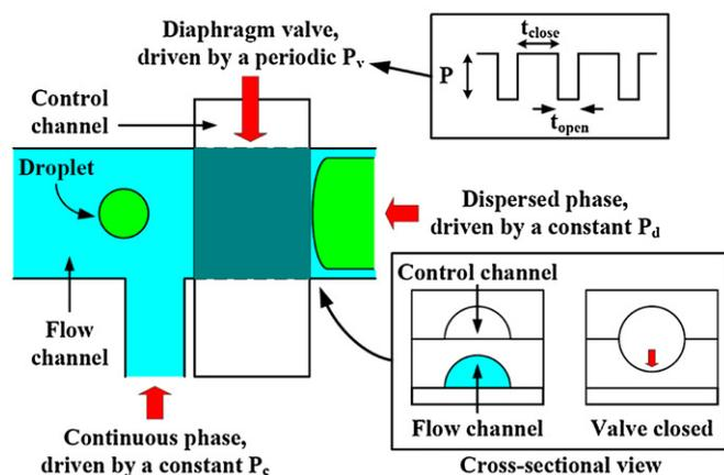
Figure 4. Schematic illustration of the proposed metering scheme.
