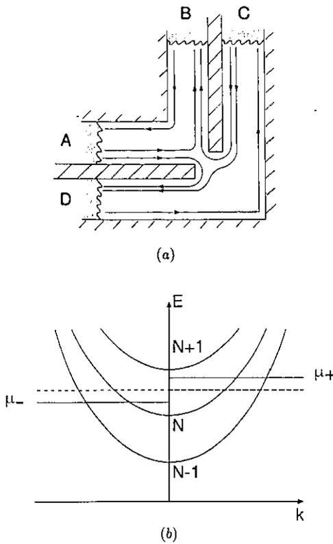
**Figure 1.** (a) Schematic diagram of the asymmetric QPC. The letters A, B, C, D refer to ohmic contacts and the lines are edge states with the arrows representing the current direction. (b) Energy against wavevector of electrons in 1D subbands of a QPC. The broken line is the equilibrium Fermi energy and  $\mu^+$  and  $\mu^-$  are the chemical potentials of the electron source and drain reservoirs respectively.
