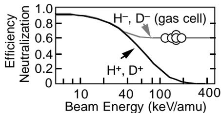
**Figure 17.** Neutralization efficiency as a function of beam energy (keV·amu<sup>-1</sup>). The solid lines are theoretical predictions and circles show the measured values for negative deuterium ions in the JT-60U experiment (Ref. [277]).
