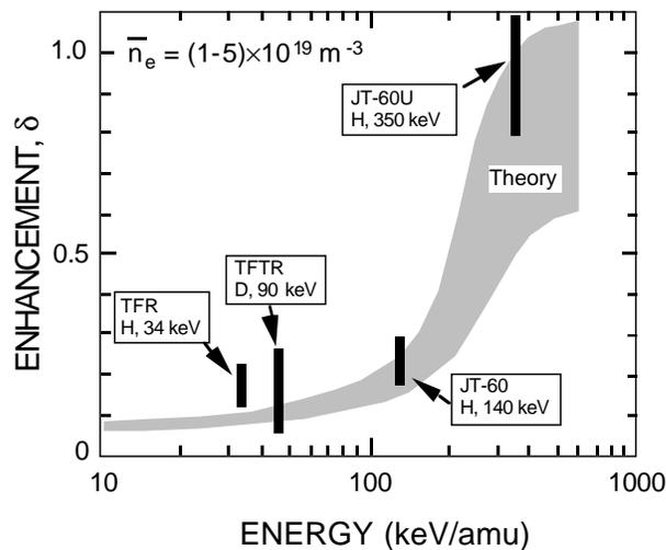
**Figure 10.** Comparison of the experimental enhancement in stopping cross-section with theory (shaded area). The spread in the theoretical curve reflects the range of values of plasma parameters ( $n_e$ ,  $T_e$ ,  $T_i$ ,  $Z_{eff}$ ), as well as the underlying energy dependence, which is indicated in the figure. For the individual experiments indicated, the appropriate values of  $T_e$ ,  $T_i$  and  $Z_{eff}$  have been taken.
