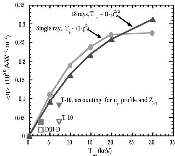
**Figure 1.** Comparison of predicted on-axis current drive and experimental results. The curves (marked by ● and ▲) are simulations showing the influence of temperature profiles and divergence of the wave due to diffractive effects. Experimental results from T-10 and DIII-D are also shown (marked by ▽ and □). Corrections for density profiles and  $Z_{eff}$  have been made for both experimental results and marked by the corresponding filled symbols (Ref. [28]).
