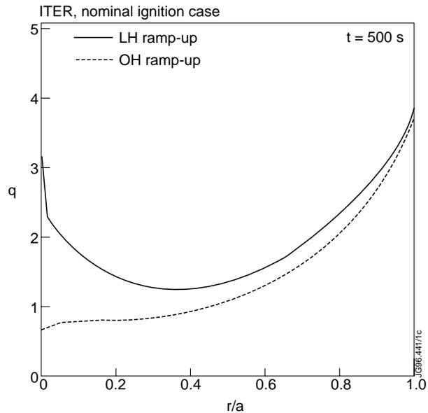
**Figure 8.**  $q$  profiles at  $t = 500$  s for simulated ohmic and LH assisted plasma current ramp up in ITER.
