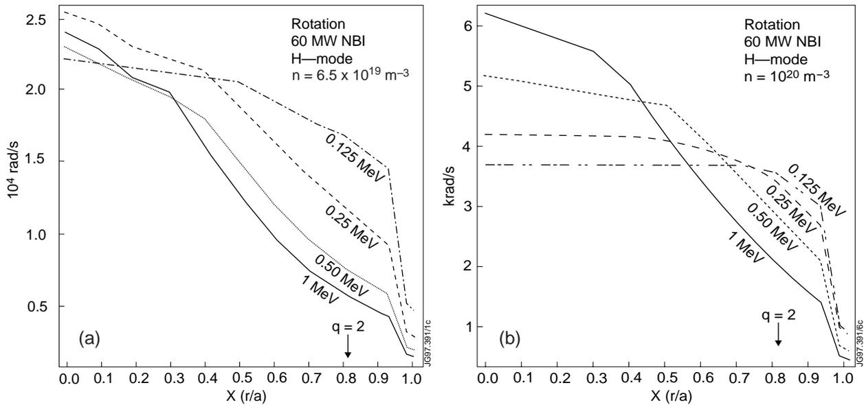
**Figure 16.** (a) Simulated toroidal rotation profiles during the density ramp along the route to ignition in ITER for an ELMy H-mode with 60 MW of NBI into a plasma with  $n_e = 6.5 \times 10^{19} \text{ m}^{-3}$ . Various beam energies from 125 keV to 1 MeV are simulated. (b) as in (a), but simulated during the flat-top density phase in ITER for an ELMy H-mode with 60 MW of NBI for  $n_e = 10^{20} \text{ m}^{-3}$ .
