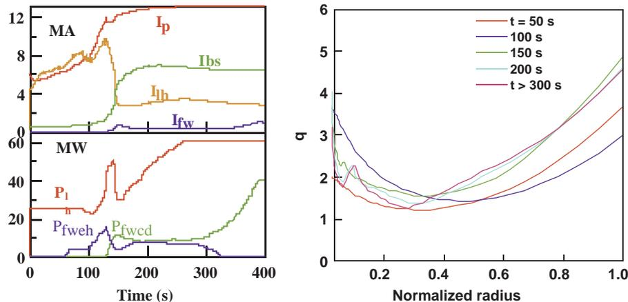
**Figure 9.** Results of a simulated ITER steady state advanced scenario showing: (left) time traces for the plasma current,  $I_p$ , bootstrap driven current,  $I_{bs}$ , lower hybrid driven current,  $I_{lh}$ , fast wave driven current,  $I_{fw}$ , lower hybrid power,  $P_l$ , fast wave electron heating power,  $P_{fweh}$ , and fast wave current drive power,  $P_{fwcd}$ ; (right) safety factor profiles at several time slices.
