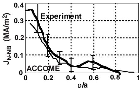
**Figure 13.** Measured and computed N-NB driven current profile in JT-60U: 2.0 MW of hydrogen N-NB (0.35 MeV) is injected into a hydrogen plasma with  $I_p = 0.6$  MA,  $n_e = 0.7 \times 10^{19} \text{ m}^{-3}$ .
