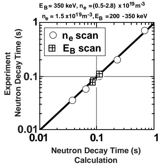
**Figure 11.** Comparison of experimental data with the theoretical prediction of the post-NBI decay time of the neutron rate during and after an N-NBI pulse in JT-60U. The calculation was made with a transport code based on classical slowing down.
