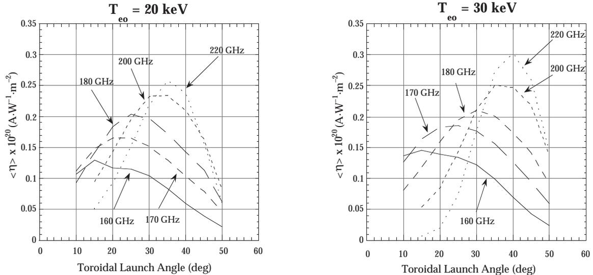
**Figure 2.** The current drive figure of merit for 24 MA, 6 T target plasmas with  $T_{e0} = 20$  keV and  $T_{e0} = 30$  keV. The figure of merit,  $\langle \eta \rangle$ , is plotted against toroidal launch angle for selected frequencies between 160 and 220 GHz (Ref. [28]). Note that these calculations were performed for an earlier version of the ITER EDA design, but the results are still, in essence, valid.
