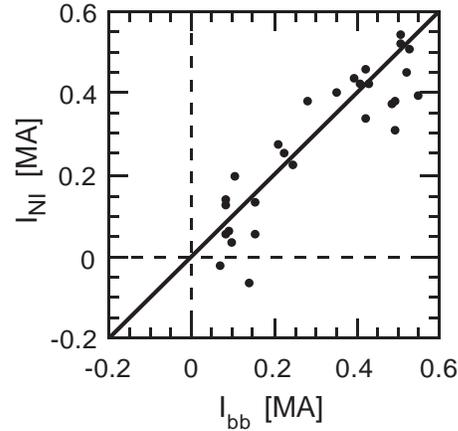
**Figure 12.** Interpreted non-inductive current,  $I_{NI}$ , versus sum of predicted (beam driven current plus bootstrap) current,  $I_{bb}$ , for several JET pulses with co-NB and counter-NB (Ref. [261]). The magnitude of the beam driven and bootstrap currents is similar, about 250 kA, in these JET discharges.
