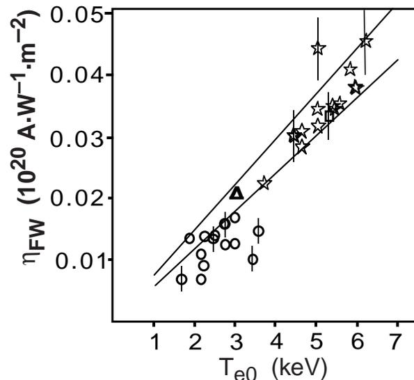
**Figure 4.** FWCD efficiency versus central electron temperature in both DIII-D and Tore-Supra experiments: circle, L-mode on DIII-D; triangle, L-mode on Tore-Supra; square, VH-mode on DIII-D; star, NCS L-mode on DIII-D. The lines are the lower and upper bounds of the simulations (ray tracing code CURRAY and full wave code ALCYON).
