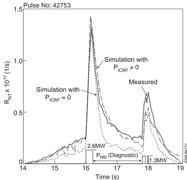
**Figure 3.** Comparison of the experimental neutron rate, in a JET DT discharge with second harmonic tritium ICRF heating alone, with simulations using PION. The two NBI pulses are diagnostic pulses for the measurement of  $T_i$  (they cause large excursions in the neutron rate because the injection energy is close to the maximum of the fusion cross-section). (From Fig. 4 in Ref. [110].)
