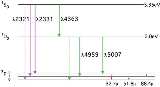
**Figure 6.** Lower energy levels and forbidden transitions for the O III ion.
