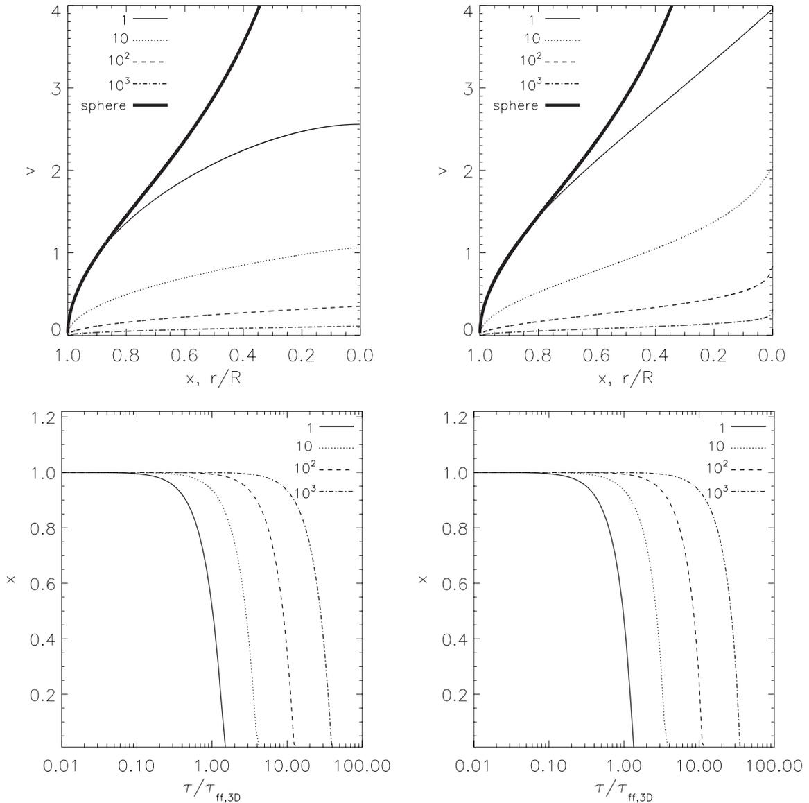
**Figure 2.** Top: evolution of the edge velocity for a filamentary cloud, compared to the corresponding velocity for a spherical cloud (thick line). Bottom: normalized position of the filament’s edge as a function of time, normalized to the spherical free-fall time estimate. Left: case 1, with  $\rho = \text{const}$ . Right: case 2, taking  $\rho(l) = M/\pi R^2 l$ . The different lines show different values of  $A$ .
