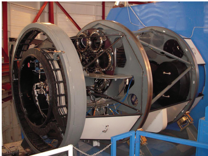
FIG. 20.—IMACS installed at the west Nasmyth platform of Baade, with most of the enclosure panels removed. This photo shows the carriage with its self-steering rollers supporting the rotation IMACS structure assembly. The rotating assembly consists of three sections. (1) Main structure—two monocoque disks (FOSS and MOSS) connected by the gray square-tube main truss. This section encloses the collimator and its baffle and the f/4 train: filter server, shutter, f/4 camera, and Mosaic-1 CCD camera (all far side, not visible). (2) Forward compartment, the short projection from the FOSS disk to the Nasmyth instrument rotator. This section encloses the field lens, the mask server, the three guiders, and the calibration unit. (3) Aft compartment—the secondary truss ( black bars ) supports the cantilevered, rotating portion of the utility wrap at the back of the instrument. In this section is the MOSS box, the weldment to which the collimator and f/2 and f/4 cameras are attached—in other words, the spectrograph. Also visible is the primary structure ( wheel ) of the disperser server; the gratings and grisms face forward and are identifiable by the index rings used to latch a selected unit to the spectrograph. Also enclosed in the aft compartment are the f/2 train: filter server, shutter, f/2 camera, and detector. The filter server and detector are slightly visible within the utility wrap.
