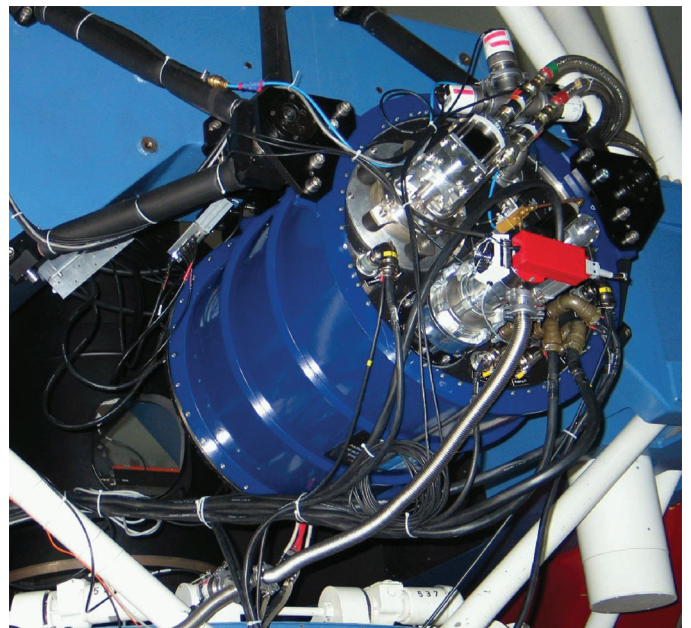
FIG. 16.—The GROND instrument at the 2.2 m telescope. Left : Grand view of the telescope, GROND to the lower left, the light baffle on top of M3 in the middle, and the main electronics rack at the top. Right : Blow-up of the GROND vessel and its various connections. The backside of the cryostat contains the CCC, the turbo-molecular pump, as well as a small emergency pump for rare cases of power outages.
