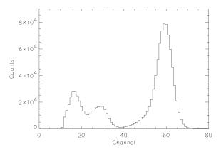
FIG. 3.—Calibration histogram of the HEXTE <sup>241</sup>Am gain control source. The data were accumulated over one day on 1997 January 10. The 60 keV gamma-ray line, the complex of Np L de-excitation lines around 17 keV, and the K-escape lines near 30 keV are evident. Each channel corresponds to approximately 1 keV.
