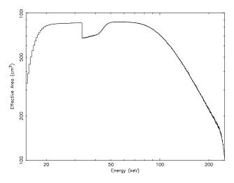
FIG. 5.—HEXTE effective area versus energy for cluster A. The reduction at lower energies is due to photoelectric absorption in the housing above the detector, while the reduction at higher energies is due to the finite NaI(Tl) thickness. The sharp drop and smooth recovery near 30 keV is due to the change in photoelectric cross section at the K edge of iodine and the onset of K-escape losses.
