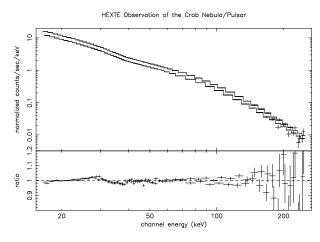
FIG. 11.—HEXTE counts histogram versus energy plus best-fit broken power-law model for fitting the Crab Nebula/pulsar spectrum in clusters A and B simultaneously. The upper plot shows the observed data plus model for each cluster with higher energy data rebinned into 10 keV groups for display only. The lower plot shows the ratio of the residuals of the best-fit model to the data.
