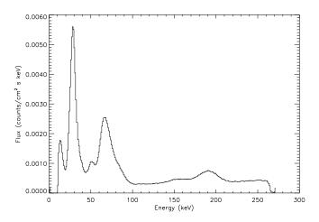
FIG. 6.—HEXTE background for a single detector plotted versus energy. Background lines due to activation of the iodine by cosmic and trapped radiation are evident at 30, 55, 66, and ~190 keV, as are the  $K_{\alpha\beta}$  lines at 74 and 85 keV from fluorescence of the lead collimator. The data are from a 7.5 hr observation of blank sky fields.
