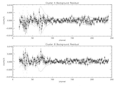
FIG. 10.—Net off-source counting rate histogram versus pulse-height channel for a  $5 \times 10^6$  s accumulation of observations with greater than 50 ks duration for the two HEXTE clusters. The detector gain is approximately 1 keV per channel, and the energy range covered is 15–240 keV. The dotted lines represent  $\pm 0.5\%$  of the background per channel.
