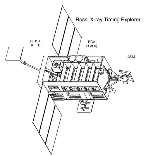
FIG. 1.—*RXTE* spacecraft viewed from above to reveal the scientific instruments. The five PCA proportional counters and the two HEXTE clusters are shown in relation to the rest of the spacecraft components, such as the two high gain antennae for communications with the ground via the tracking and data relay satellite system, the two solar-power arrays that can rotate to face the Sun, and the ASM on the end with clearance to view the sky.
