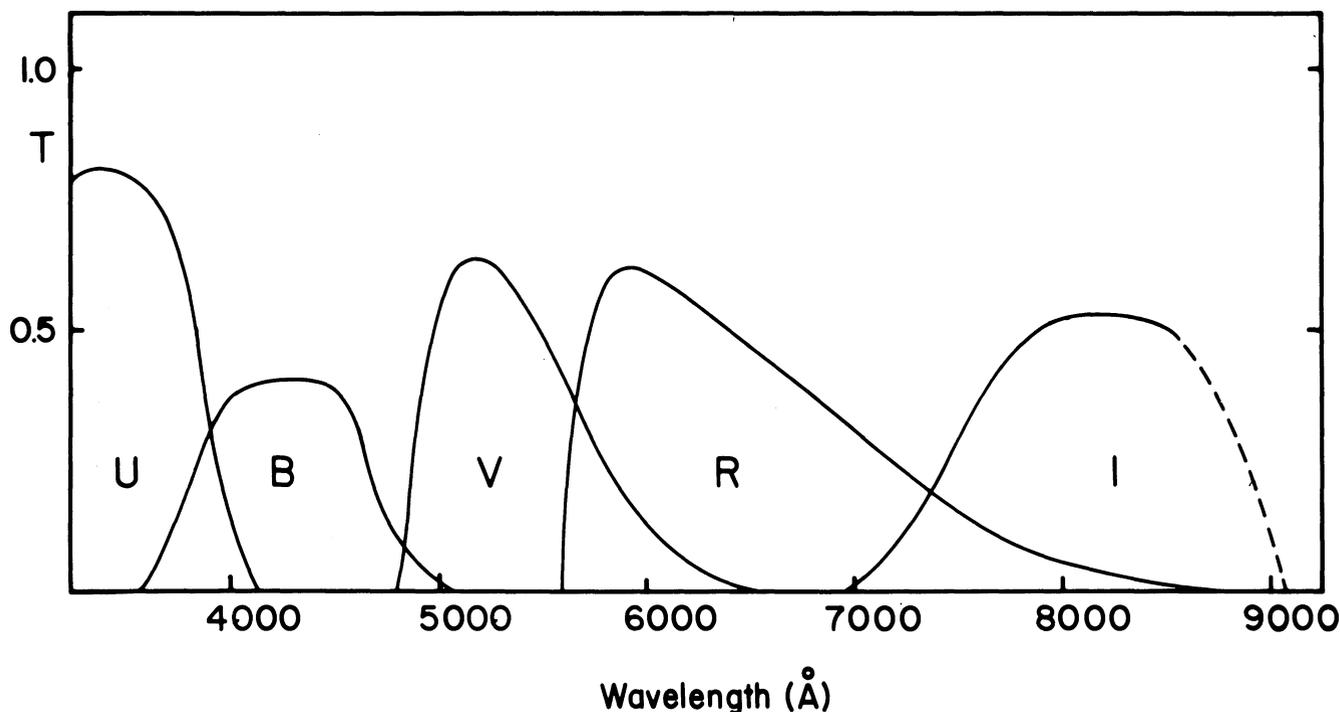
FIG. 1.—Transmission curves are shown for the *U*, *B*, *V*, *R*, *I* filter combinations used in this program. They were measured with the Oriel spectrometer at CTIO. The long wavelength cutoff of a typical RCA 31034 photomultiplier is shown as a dashed curve.
