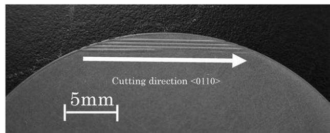
Fig. 4. Sapphire surface after cutting by commercial dicing blade. Commercial dicing blades generate meandering lines and are broken only by 50 mm of cutting length in  $\langle 01\bar{1}0 \rangle$  direction.
