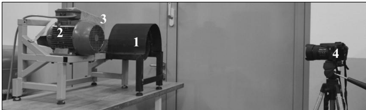
Figure 2. Experimental setup for the spinning experiments (1, mold; 2, engine; 3 gear; 4, high-speed camera).
