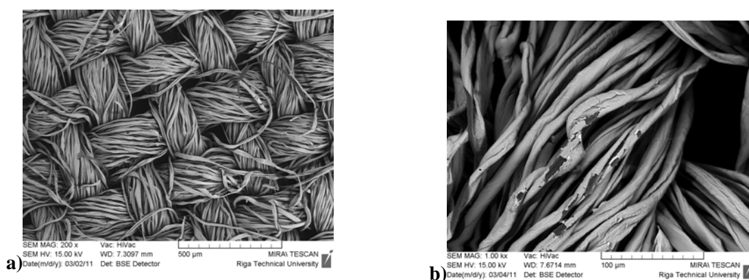
Figure 5. Micrograph of sample coated with copper by vacuum evaporation technology a) before and b) after washing
