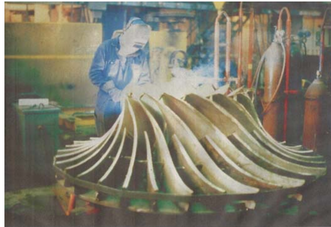
Fig. 5 A splitter blade runner during fabrication around 40 years ago.
