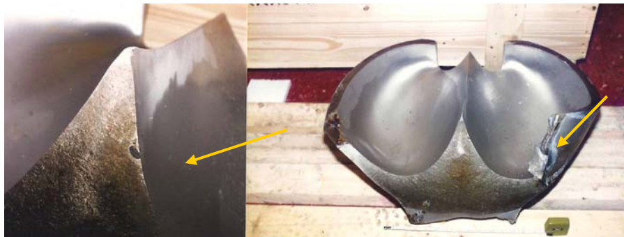
Fig. 8 Broken Pelton bucket caused by a not successful not heat treated small weld repair. Detail to the left.
