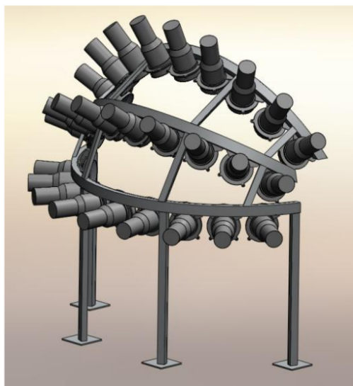
Figure 2. Arrangement of 27 liquid scintillators, which constitute half of the array. The neutron detectors will be 1.0 m from the fission chamber. The array of {}^6\text{Li} -glass detectors will be smaller in number and will be at a flight path of 40 cm from the fission source.
