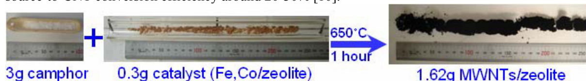
Fig. 2 Optical photograph of camphor and zeolite bed before and after CVD.
