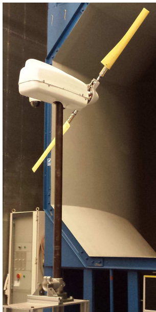
Figure 1. Small-scale two-bladed wind turbine
