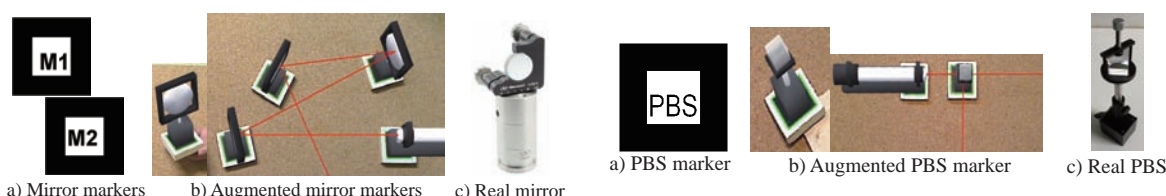
Figure 8. Mirror markers and augmented mirror markers. Figure 9. PBS marker and augmented PBS marker.
