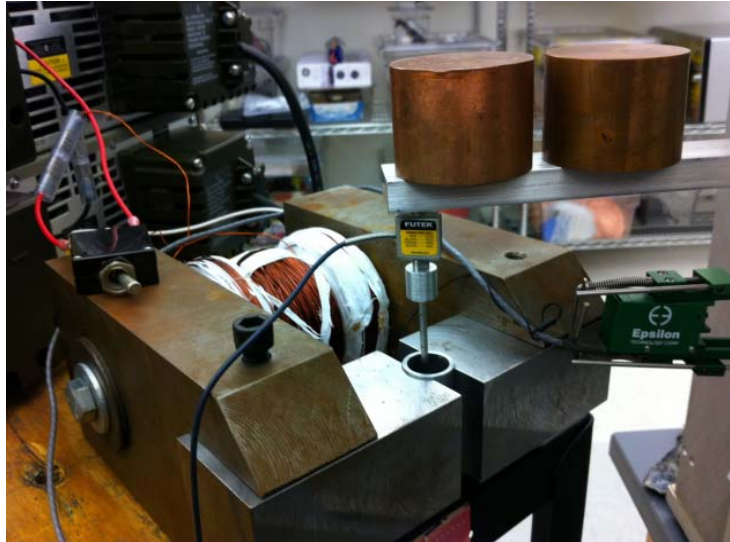
Figure 4. Photograph of the setup by which the compression tests were performed.
