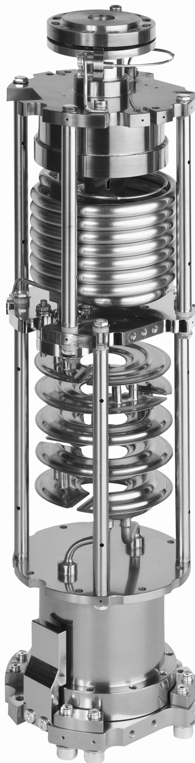
Figure 2. The UHV compatible dilution unit. The pre-cool heat switch strike-plate can be seen at the bottom left of the image.
