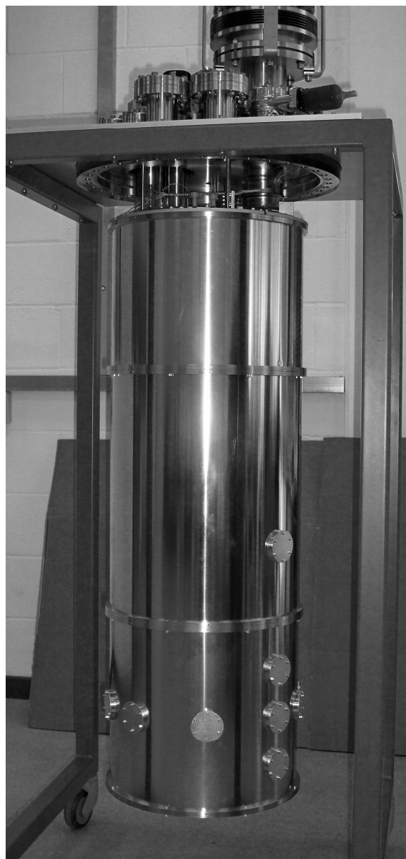
Figure 6. The system with the OVC removed showing some of the optical ports in the PT1 shield.
