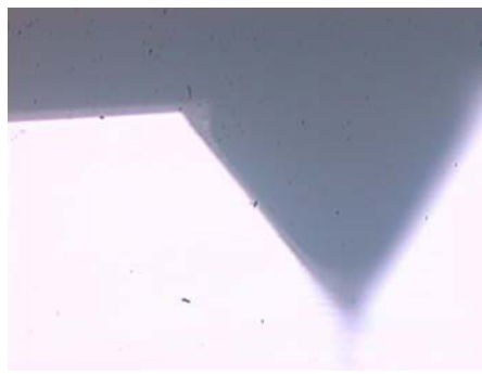
Figure1. Photoresist coverage of a via-hole
